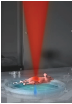
Trans-illumination for 3D fluorescence tomography.
